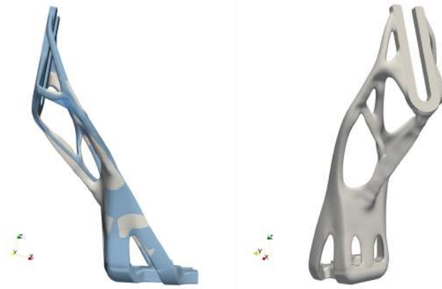
Figure 1: Additive Manufacturing: Overhang-free shape for an attachment structure. In transparent blue is the initial shape, and in grey the final shape .
